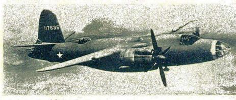
FULL FEATHER POSITION of the propeller on a B-26. In this position propeller blades of an inactive engine are parallel to direction of flight.
