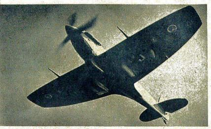
CLIPPED WINGS characterize Spitfire V. These eliminate drag, thus increasing speed. Plane is less maneuverable, due to more wing loading.
