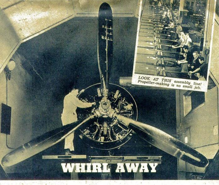
GIANT PROPELLER DESIGNED for bombers and troop transports which must brave the stratosphere. This picture shows the world's very largest propeller undergoing stringent tests in the testing chamber.
