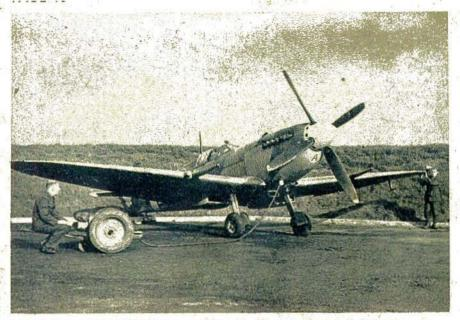
SPITFIRE WARMING UP for take-off. The improved Spitfire now in service has four-bladed propellers and a radiator under eact wing.
