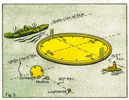
A pelorus is an instrument for taking hearings (determining the direction) of an object external to the plane for purposes of location. Usually the compass is under cover and one cannot see over it to get bearings. The pelorus is really a dumb compass mounted somewhere near the magnetic compass with its fore-and-alt line parallel to the plane's center tine on which the compass is located and in such a position that one can see objects outside the ship across the pelorus dial.
