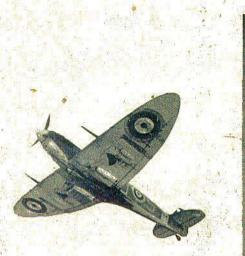
SPITFIRE V with two 20 mm. cannon, four machine guns in wings.
