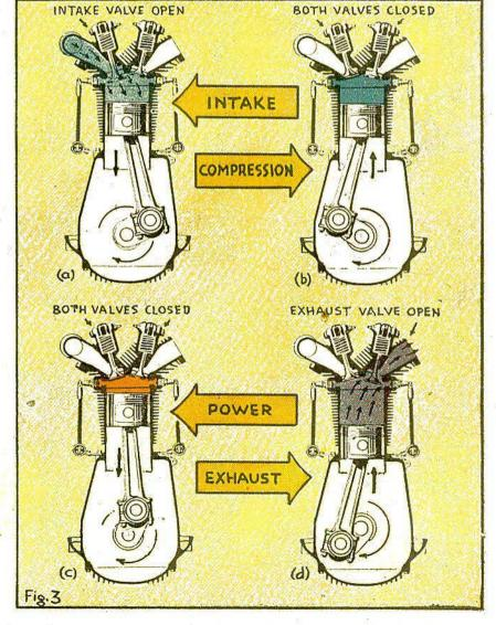
Almost all aircraft engines operate on the four-stroke cycle principle. Each stroke is one vertical movement up or down of the piston. (See Fig. 2). Each cycle requires one revolution or two strokes of the piston, one up and one down, so that two revolutions or two cycles require four strokes. Some diesel engines and modern airplane gas engines utilize the two-stroke cycle so that only two strokes or one revolution of the crankshaft are required for a complete cycle of operation.
