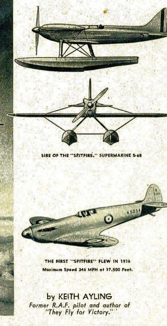
ted with a three-blade, variablepitch propeller, the second model Spitfire became the standard single seater fighter of the R.A.F. Powered by a Rolls-Royce 12cylinder Merlin, giving a maximum of 1,030 h.p. at 16,250 feet, it was credited with a speed of 367 m.p.h. at 18,000 feet.
