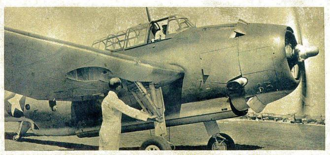
"CLOSE BOMB BAY DOORS" is what Mechanic Roland Wentzel, with an upsweep of the hands, is telling the man in the plane. The men are ground-testing the engine of this Grumman Avenger torpedo bomber.
