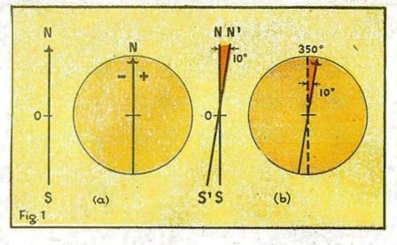
If a bar or similar magnet be suspended at its balance point it will take up a general north and south direction in the plane of the lines of force of the earth's magnetic field, or, more simply, in the plane of the magnetic meridian. This, then, is the working principle of the mariner's magnetic compass. The northseeking end of the compass points toward magnetic north, being attracted toward the magnetic north pole and the south-seeking end points toward the magnetic south pole.
