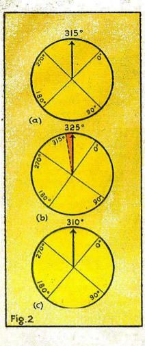
left to a reading of 325°; we have then allowed for the fact that a deviation of 15° E draws the magnetic reading of the card to the right to a reading of 310°. Consequently, the pilot knows that to steer a true course of 315° he should steer a compass course of 310°.
